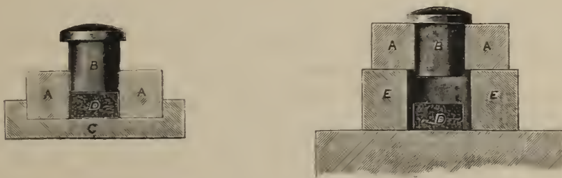
FIGS. 7 AND 8. METHOD OF COMPRESSING PLUMBAGO POWDER
